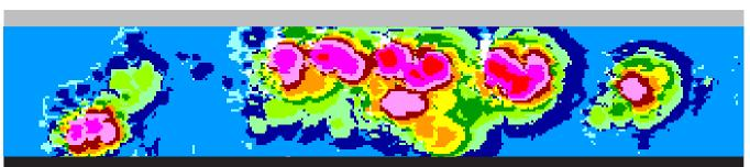
Time of Flight Diffraction Inspection for Weld Flaw Detection and Sizing
